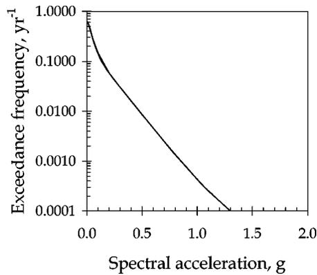
Figure 5. Seismic hazard function for a Los Angeles site.
