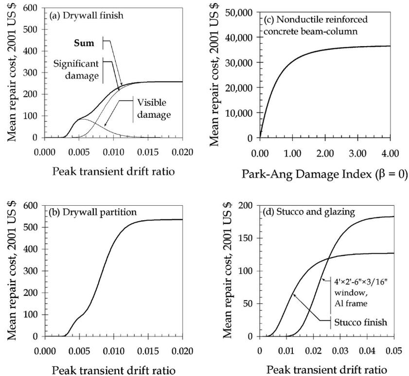
**Figure 1.** Mean assembly vulnerability functions for five assembly types (d shows two to save space).
