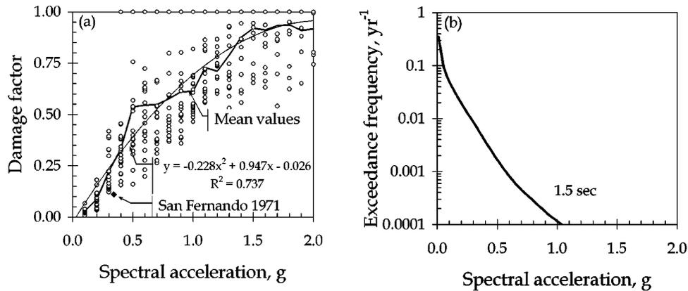
**Figure 2.** (a) Mean seismic vulnerability function, and (b) site hazard function for Van Nuys building.
