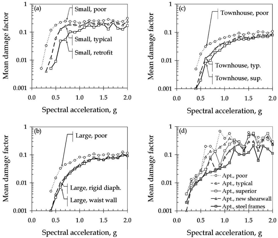
Figure 4. CUREE-Caltech Woodframe Project mean vulnerability functions.
