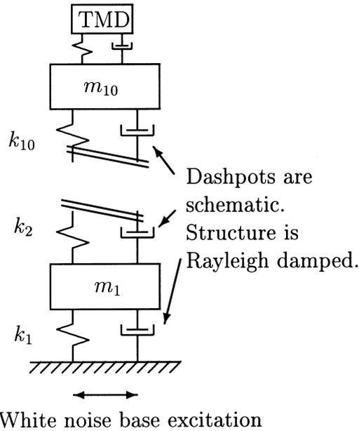
Fig. 3. 10-DOF shear building model with TMD.
